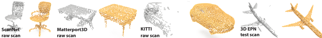
Figure 1: We present a point-based shape completion network that can be directly used on raw scans without requiring paired training data. Here we show a sampling of results from the ScanNet, Matterport3D, 3D-EPN, and KITTI datasets.
