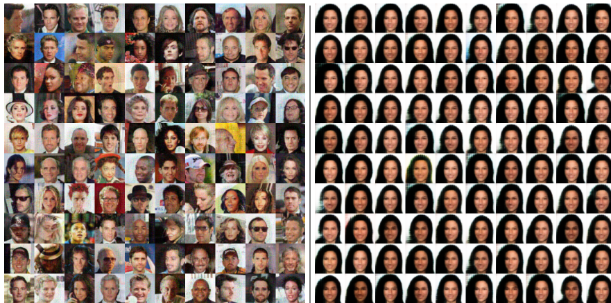
Figure 20: L_2 Optimization Latent Attack on CelebA Dataset (single latent vector target): Adversarial examples generated for 100 images from the CelebA dataset (left) and their VAE-GAN reconstructions (right).
