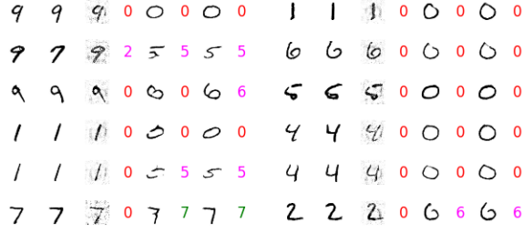
Figure 4: Results for the L_2 optimization latent attack on the VAE-GAN, targeting the mean latent vector for 0. Shown are the first 12 non-zero images from the test MNIST data set. The columns are, in order: the original image, the reconstruction of the original image, the adversarial example, the predicted class of the adversarial example, the reconstruction of the adversarial example, the predicted class of the reconstructed adversarial example, the reconstruction of the reconstructed adversarial example (see Section 4.5), and the predicted class of that reconstruction.
