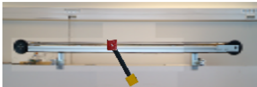
Figure 3: A frame captured by the differentiable camera looking at the model of the pendulum-cart system. The resolution used is 288 by 96 pixels. All the textures are made from pictures of the actual system.
