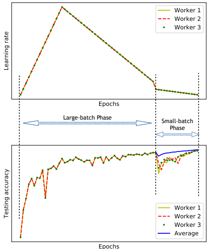
Figure 1: Learning rate schedules and CIFAR10 test accuracies for workers participating in SWAP. The large-batch phase with synchronized models is followed by the small-batch phase with diverging independent models. The test accuracy of the averaged weight model is computed by averaging the independent models and computing the test loss for the resulting model.
