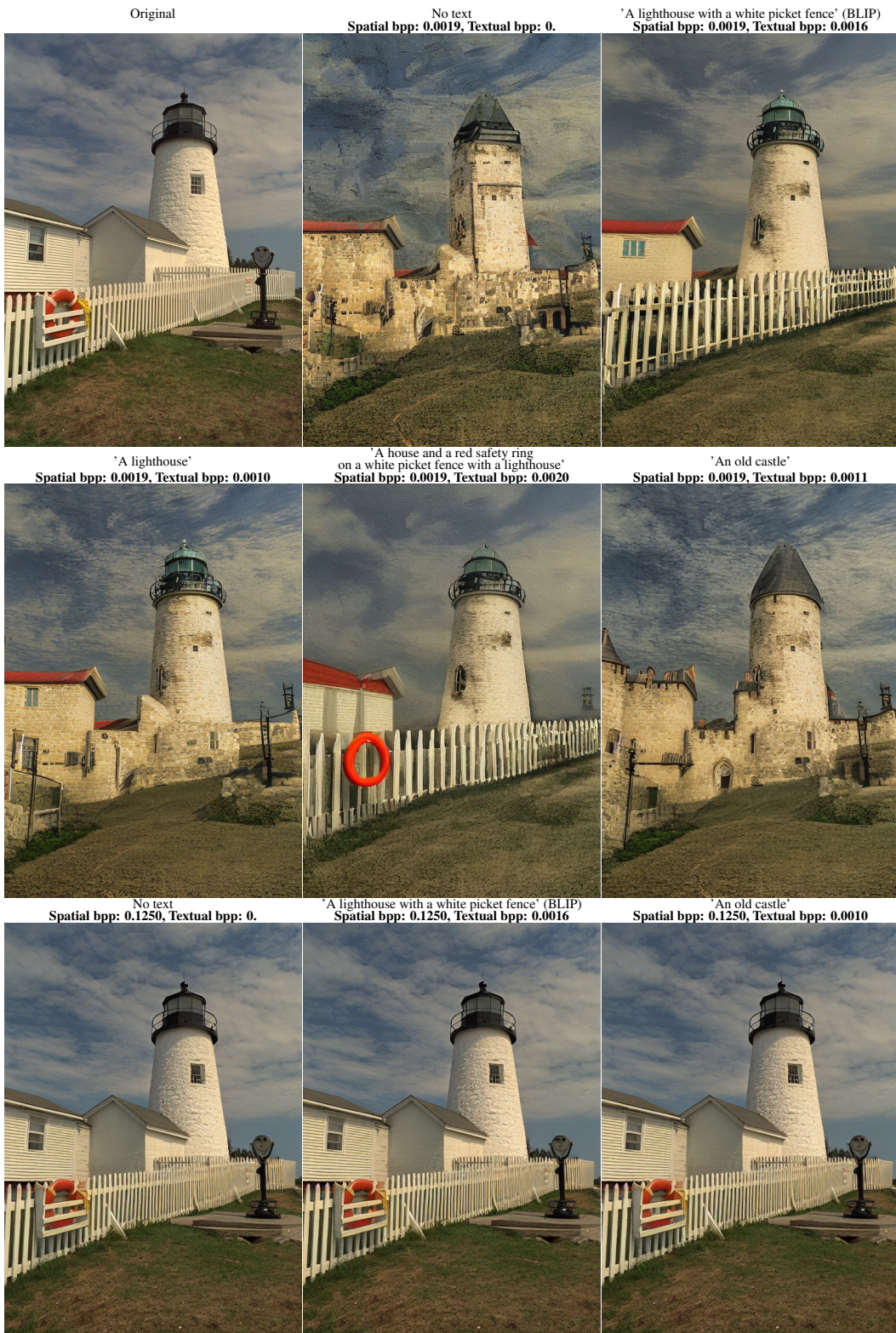
Figure 12: Reconstructions of a Kodak image when varying the global textual conditioning with a spatial bpp of 0.0019 (first two rows) and 0.1250 bpp (last row). Samples with the same spatial bpp are reconstructed from the same initial Gaussian noise from the same model.
