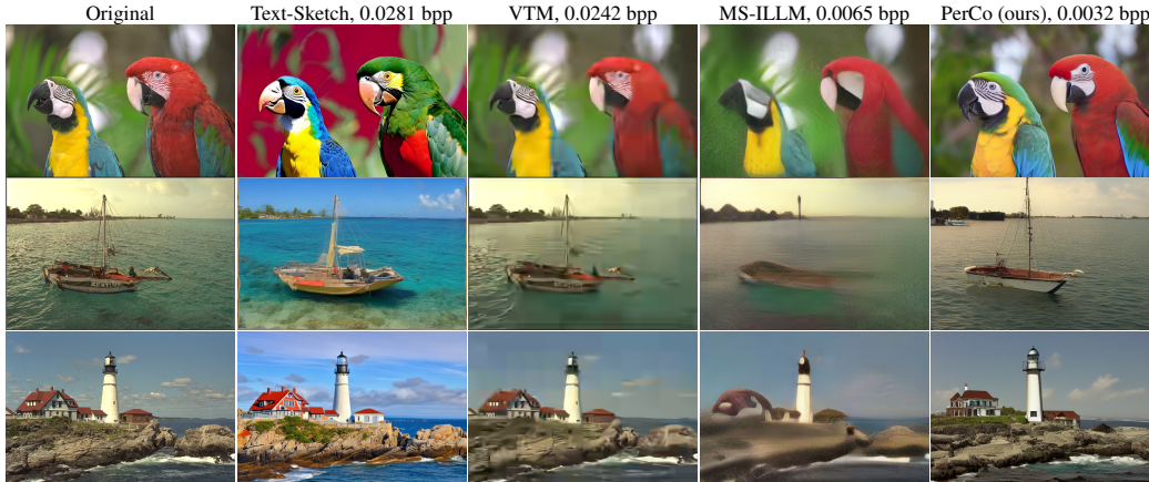
Figure 1: Kodak images compressed with the diffusion-based Text-Sketch approach PICS (Lei et al., 2023), the hand-crafted codec VTM (vtm), MS-ILLM (Muckley et al., 2023) which leverages an adversarial loss, and with PerCo (ours). Taking the lowest available bitrate for each method.
