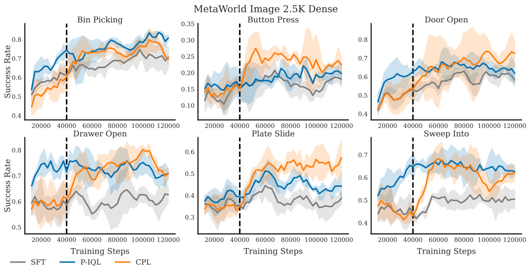
Figure 5: Image-based results in MetaWorld with 2.5K segments and dense comparisons. This plot additionally shows the CPL BC variant. The dotted vertical line indicates when BC pretraining stops for CPL and SFT.
