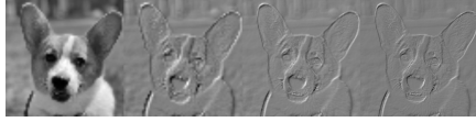
Figure 2: A Laplacian pyramid hierarchy with S = 4 . Left to right: z^{(1)}, \dots, z^{(4)} .
