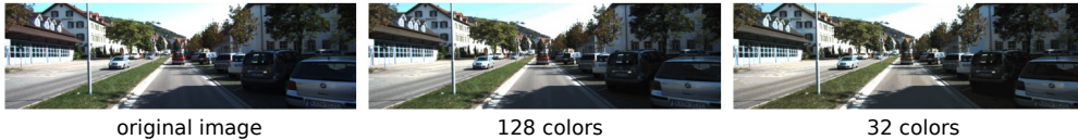
Figure 3: Color quantization. We apply K-Means algorithm to cluster RGB pixel values into discrete bins. The resulting image with 128 bins is hardly distinguishable from the original image by human eyes.
