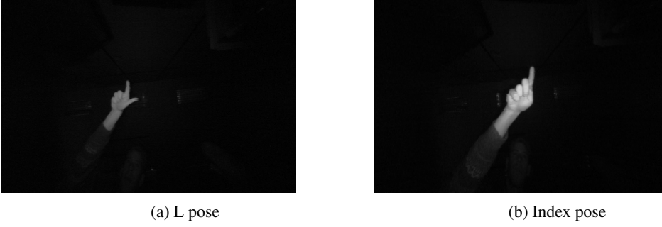
Figure 19: Examples of the original images of the considered hand-gestures. We recognize the "L"-sign in Figure 19a and the index sign in Figure 19b. Observe that the near-infrared images highlight the hand pose well and blends out much of the non-useful or noisy background.
