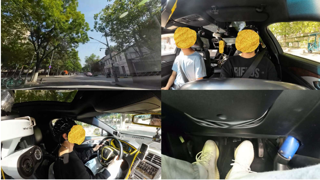
Figure 1: Example Snapshots of the Video Modalities: top left – Baseline (forward road view); top right – Driver1 (driver’s face view); bottom left – Driver2 (driver’s posture view); bottom right – Driver3 (driver’s feet view).
