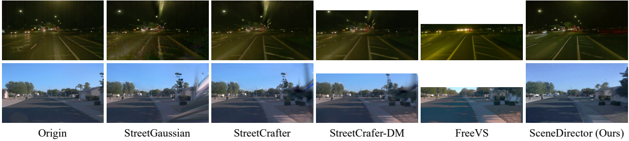
Figure 10. Qualitative comparison of Fixed Offset trajectory editing. We compare methods under a constant lateral shift trajectory in both night (top) and day (bottom) scenarios. Baselines: StreetGaussian and StreetCrafter show noticeable rendering distortions. Ours: SceneDirector successfully reconstructs full-frame, photorealistic video with precise structural alignment, effectively hallucinating plausible details in occluded regions.
