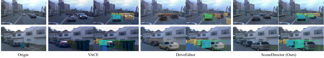
Figure 9. Qualitative evaluation of editing precision via 3D object detection. The leftmost column displays the original scene, followed by the editing results from VACE , DriveEditor , and SceneDirector . Top Row: A complex combination of object insertion and repositioning (movement). Bottom Row: Simultaneous object insertion and replacement. Legend: Filled semi-transparent boxes indicate the detection results from the perception model, while hollow wireframe boxes represent the target Ground Truth (GT) layout. Analysis: Baseline methods suffer from severe “hallucinations” (numerous false positive boxes in empty areas) and geometric misalignment (detection boxes drifting away from GT). In contrast, SceneDirector achieves precise alignment between detections and GT constraints with minimal artifacts, proving its capability to generate functionally valid data for perception training.
