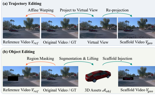
Figure 3. Pipeline for self-supervised pair construction. (a) Trajectory: We synthesize a misaligned V_{ref} via affine warping, and generate V_{geo} via round-trip projection to mimic sparsity artifacts. (b) Object: We mask targets in V_{ref} to prevent shortcut learning, while composing lifted 3D assets into V_{geo} for structural guidance.
