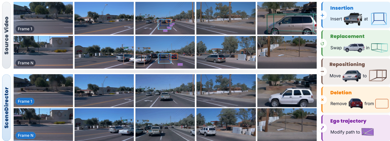
Figure 1. SceneDirector is a unified framework for multi-view driving video editing. It enables simultaneous 3D box-defined object editing (insertion, deletion, replacement, repositioning) and ego-trajectory editing in a single inference pass. By bridging geometric guidance with generative priors, it reconciles photorealistic synthesis for object editing and structural consistency for trajectory control.
