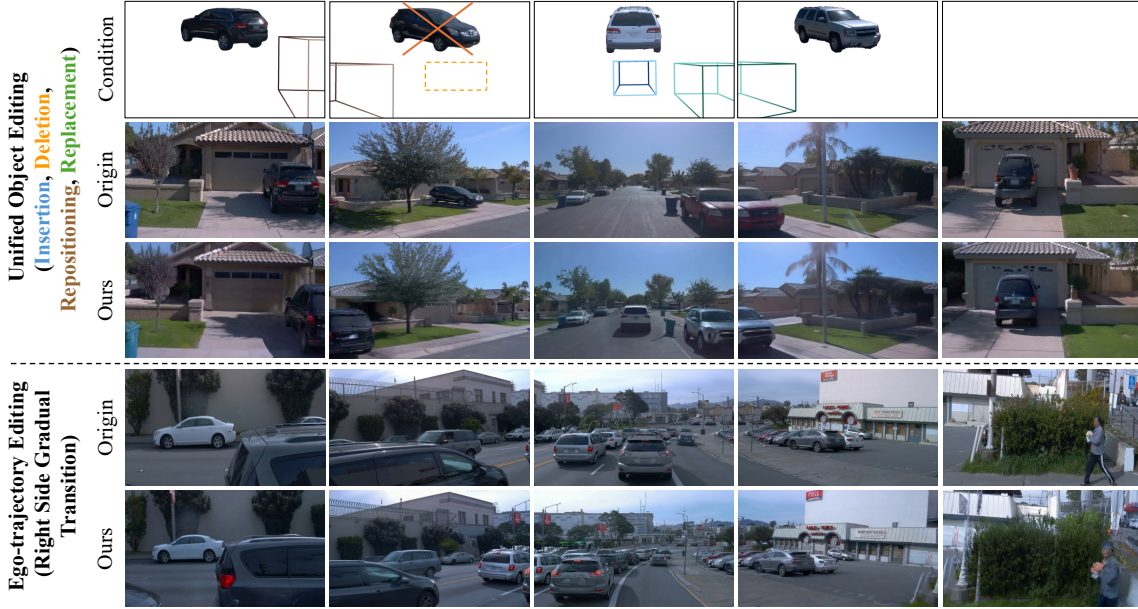
Figure 6. Qualitative results of SceneDirector on multi-view editing. Top (Object Editing) : Rows display inputs (object assets, 3D bounding boxes), source frames, and our editing results. Our method enables unified editing in a single inference pass. Bottom (Trajectory Editing) : Results under a gradual right shift demonstrate that our method preserves cross-view structural consistency and photorealism.
