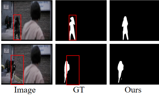
Figure R1: When the motion of an instance is too large (the instance in the red box) to accurately capture the trajectory, the saliency of the instance is often high due to the high feature contrast between them.
