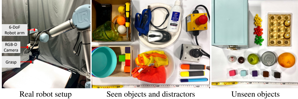
Figure 5: Real robot experiment. The figure shows our physical robot setup along with both seen and unseen objects. Seen and unseen colored blocks are also included.
