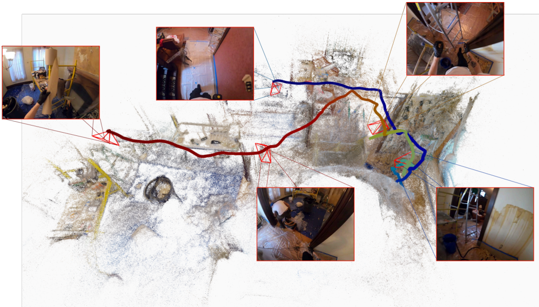
Figure 8: Visualisation of the 3D reconstruction for one video of the Ego4D dataset capturing building and refurbishment activities, with camera estimated using the EPIC Fields pipeline
