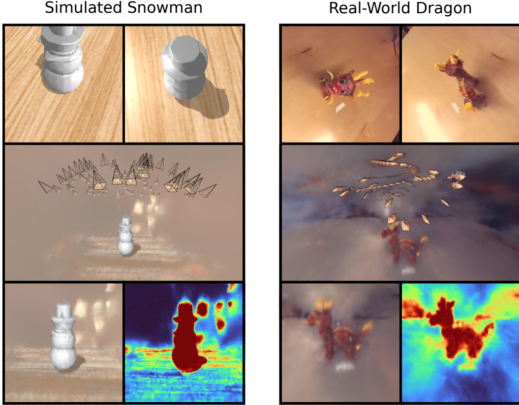
Figure 12: Comparison between NeRFs trained on simulated snowman data and real-world dragon data, which demonstrates the qualitative similarity between the two NeRFs. First row: two of the RGB images used for NeRF training. Second row: Camera poses used for NeRF training. Third row: NeRF-rendered RGB image and accumulation image.
