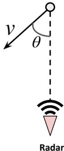
Figure 1: Target’s motion relative to the Radar’s line-of-sight axis.
