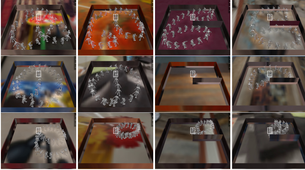
Figure 3: Trajectory visualisation for the learned agents. Top: vision agent. Middle: pose agent. Bottom: blind agent. The two left examples are tested with additional wall to observe the reaction of the robot. The white square highlights the start position. Spacing between robot snapshots is 1 s.
