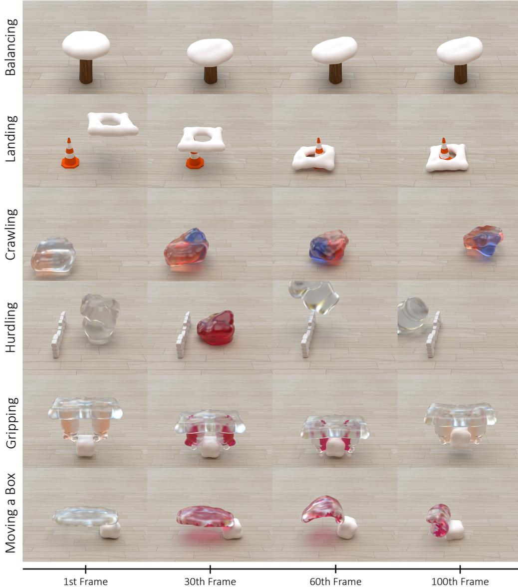
Figure 9: Examples of robots bred by DiffuseBot to achieve the all presented tasks.
