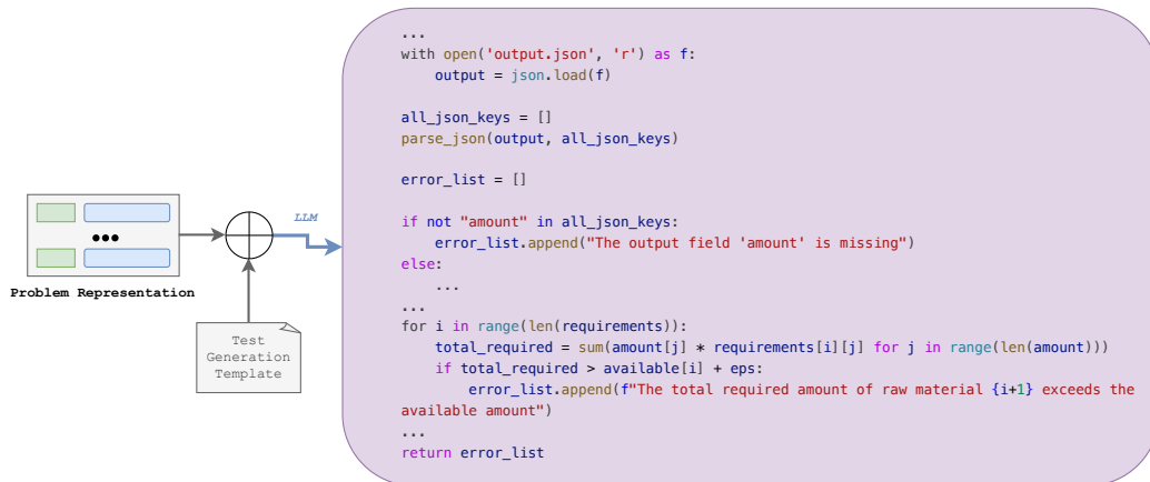
Figure 4: LLM can be used to generate tests and check the correctness of the output. After feeding the problem to an LLM using the test generation template, the model generates a script that checks the correctness of output (constraint satisfaction, output format, etc.) and returns appropriate error message if it finds a problem. The error message is used to automatically fix the code.
