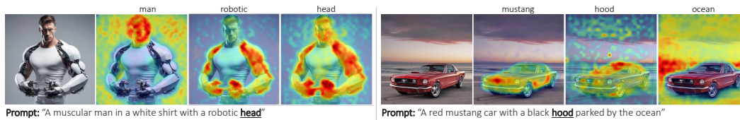
Figure 2: A visualization for the cross-attention maps of SDXL (Podell et al., 2024) that corresponds to different words of the textual prompt. Object parts such as “head” and “hood” are not well-localized, indicating that the model lacks a sufficient understanding of these parts.
