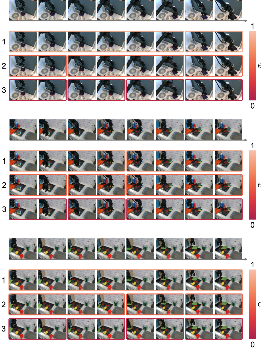
Figure 7: Multi-granular task decomposition through concept latent clustering. Visualization of sub-processes derived by clustering manipulation concept latents at different coherence thresholds ( \epsilon ) for push-and-sweep tasks (attaching an object and sliding it to another location). Higher \epsilon values (top rows) produce coarser decompositions, while lower values (bottom rows) yield finer-grained segmentation. The emergent sub-processes naturally align with semantic task components. For the third push-and-sweep-green-cloth example: the 1st sub-process of row 1 corresponds to “pressing and sliding the cloth”; the 2nd sub-process of row 1 corresponds to “releasing the cloth”; the 1st sub-process of row 2 corresponds to “positioning and pressing on the cloth”; the 2nd sub-process of row 2 corresponds to “sliding the cloth”; the 1st sub-process of row 3 corresponds to “aligning the gripper with the cloth”; the 2nd sub-process of row 3 corresponds to “pressing on the cloth”.
