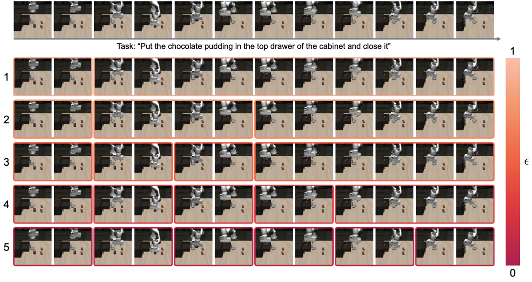
Figure 2: Multi-granular task decomposition through concept latent clustering. Visualization of sub-processes derived by clustering manipulation concept latents using Eq. 4 at different coherence thresholds ( \epsilon ) for the task “Put the chocolate pudding in the top drawer of the cabinet and close it” . Higher \epsilon values (top rows) produce coarser decompositions, while lower values (bottom rows) yield finer-grained segmentation. The emergent sub-processes naturally align with semantic task components. For example, the 3rd sub-process of row 3 corresponds to “transitioning the chocolate pudding above the top drawer”; the 4th sub-process of row 4 shows “releasing the chocolate pudding”; the 5th sub-process of row 4 represents “closing the top drawer”; the 5th sub-process of row 5 illustrates “reaching the handle of the top drawer”; the 6th sub-process of row 5 corresponds to “pushing the top drawer closed”.
