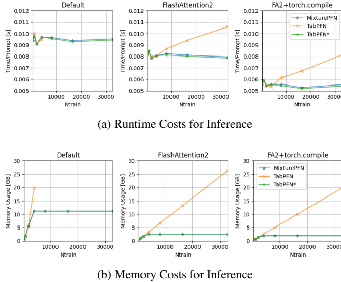
Figure 4: Computation Costs for attention compute with different hardware optimizations.
