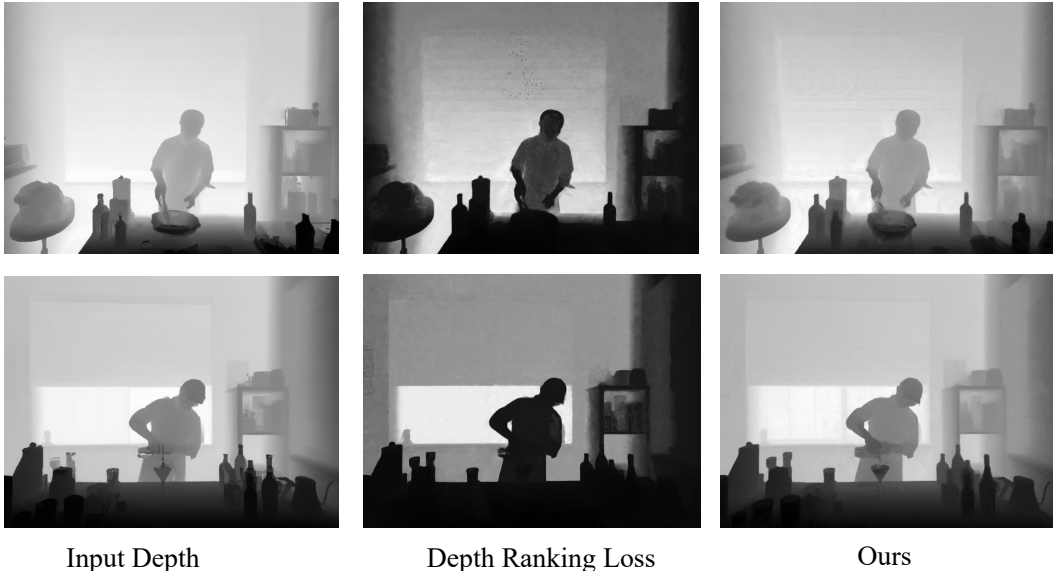
Figure 12: A visual comparison of rendered depth maps between using depth ranking loss (Wang et al., 2024b) and our ordinal depth loss.
