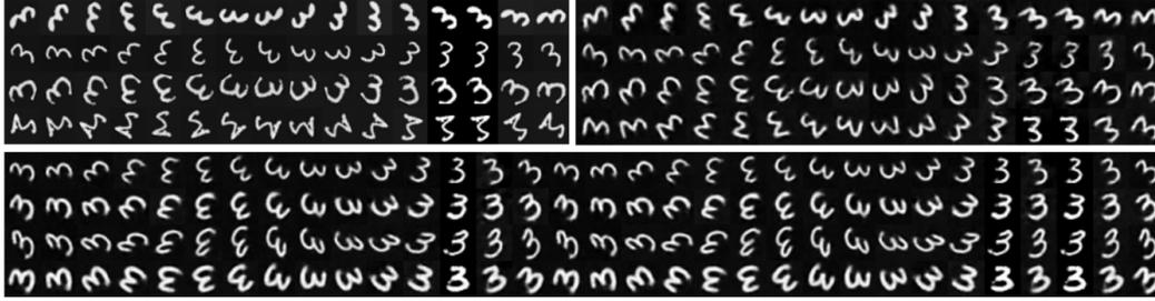
Figure 5: Results on Rotating MNIST with a learnable Hamiltonian operator. On the top left, we have four input sequences, and on the right, their reconstruction; on the bottom, we have four sequences generated by an action of Hamiltonian on the state space coordinate of the frame in the first column.
