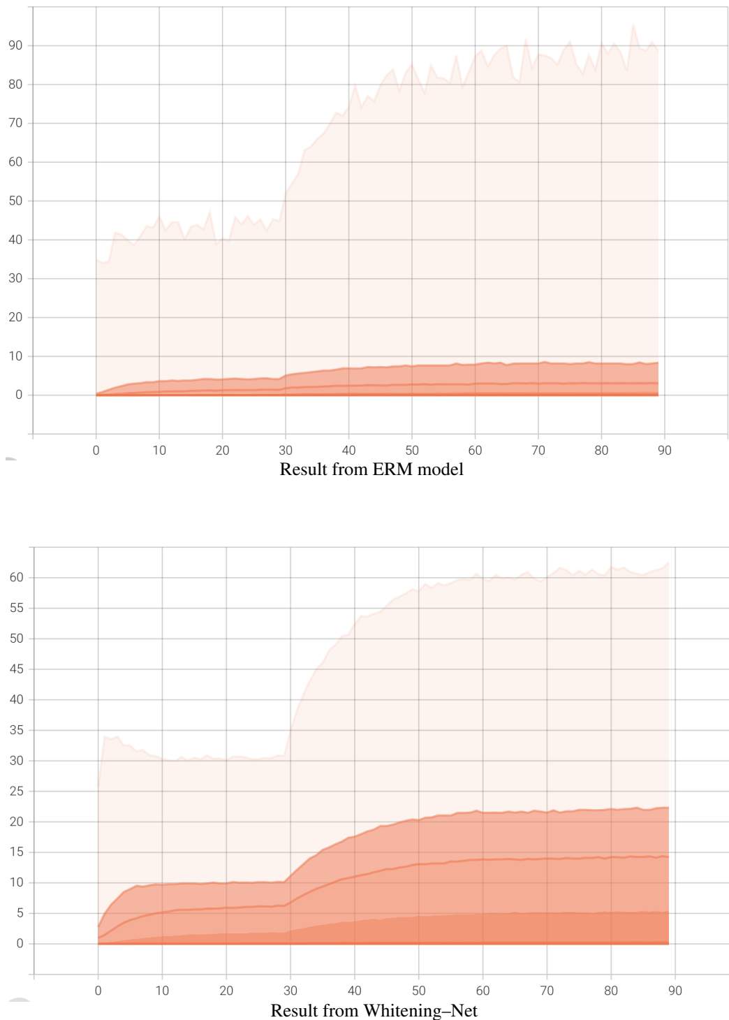
Figure 6: Singular value distributions of features fed into the classifier. The experiments are constructed on iNaturalist-LT dataset using ResNet-10 . x -axis stands for number of epoch, y -axis is the singular value. The curves from the top to the bottom are maximum-value, 99.7% quantile, 95% quantile, 68% quantile and the minimum-value, respectively. The result in top figure shows that when trained with ERM, more than 95% of the singular values are smaller than 10. In contrast, we can see that when trained with Weighting-Net, the learned features have more large-valued singular values, implying that the features are effectively decorrelated.
