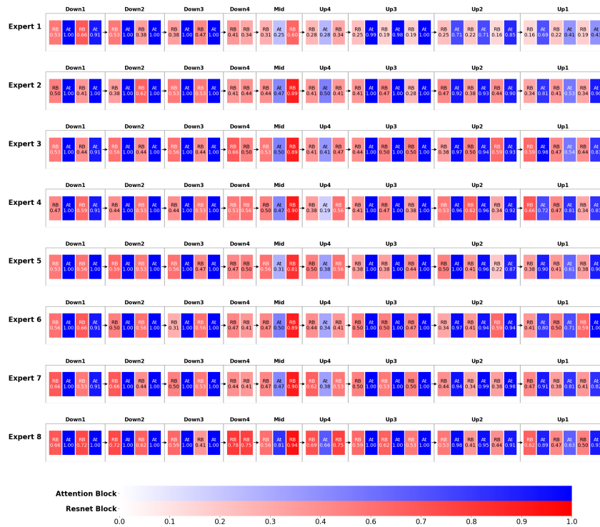
Figure 12: The block-level retained MAC ratio of the UNet architecture of all experts of APTP-Base applied to Stable Diffusion 2.1 with COCO as the target dataset. The groups of ResBlocks and the heads of Attention Blocks are pruned based on the outputs of the architecture predictor. The intensity of the color of each block represents the resource utilization of it. The number in each block indicates the precise ratio of retained MACs of the block. Conv_in, Conv_out, and skip connections between corresponding down and up blocks are omitted for brevity.
