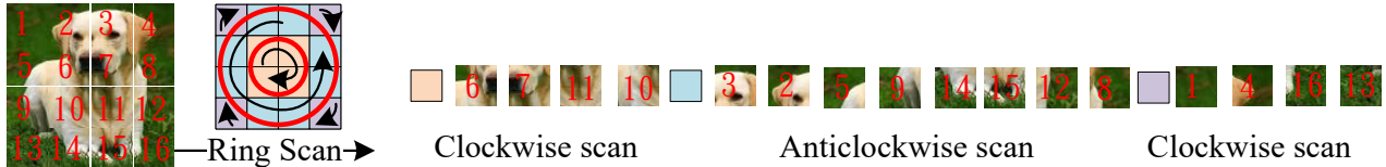
Figure 3. Ring Scan. Pixels are partitioned into concentric rings, which are interactively traversed in a clockwise or counterclockwise sequence. The resulting features are then aggregated in an order-independent fashion, proceeding from inner to outer rings.
