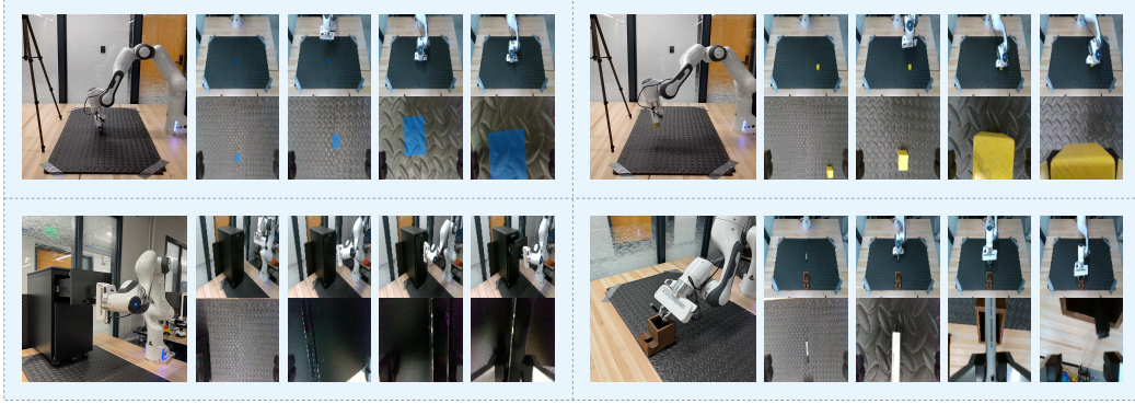
Figure 7: We deploy LaNE on four tasks with the Franka Panda robot: reach a fixed location, lift a block, open a drawer, and insert a pen. The RL agent observes two RGB images, one in front of the robot and one on its wrist. Trained from scratch, the robot achieves a 10/10 evaluation success rate with only a few demonstrations and less than one hour of learning.
