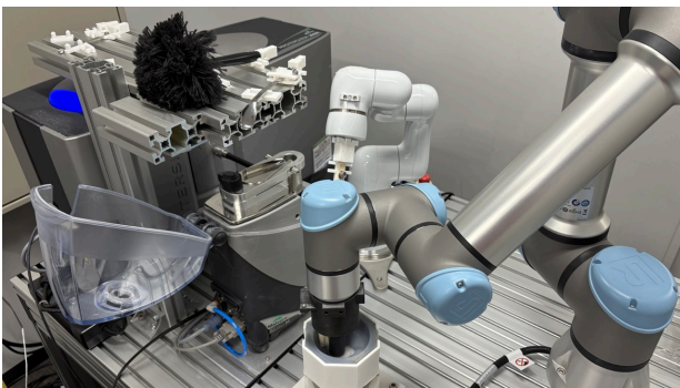
Fig. 1: Overview of the autonomous grinding system
