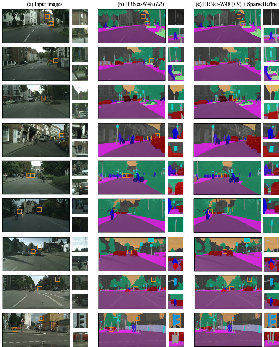
Figure A2: SparseRefine improves the low-resolution ( LR ) baseline with substantially better recognition of small, distant objects and finer detail around object boundaries.
