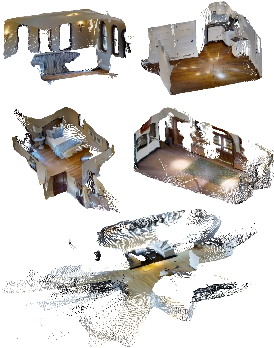
Figure 1: 3D geometry of Matterport3D using matches and certainties produced by EDM. These point clouds result from spherical triangulation with estimated poses between two omnidirectional images.
