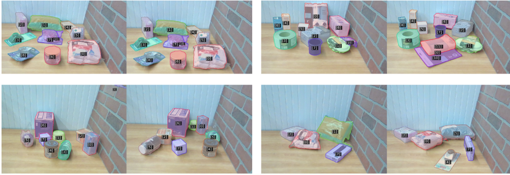
Figure 5: Failure cases on the tabletop dataset. Top left: under segmentation. Top right: over-segmentation. Bottom left: false positive (object mismatch). Bottom right: false negative (treat an existing object as new object)
