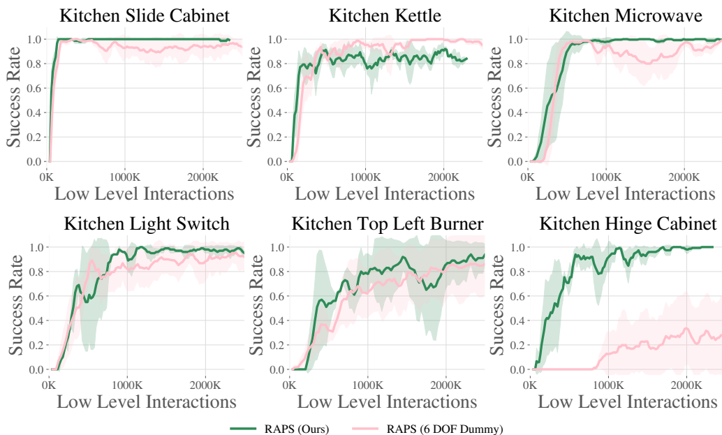
Figure 15: We plot the results of running RAPS with a 6DOF control dummy primitive, and find that in general, the performance is largely the same.
