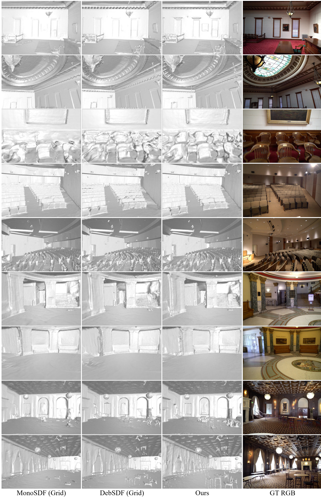
Figure 18: Qualitative Comparison on Tanks & Temples. We compare ND-SDF with previous state-of-the-art indoor implicit reconstruction methods.
