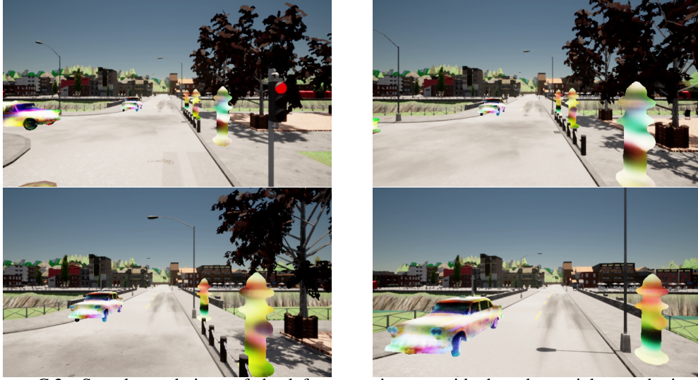
Figure C.2: Sample renderings of the left turn trajectory with the adversarial perturbations in CARLA from the ego vehicle's point of view. Four different snapshots from the evolution of the trajectory are shown.
