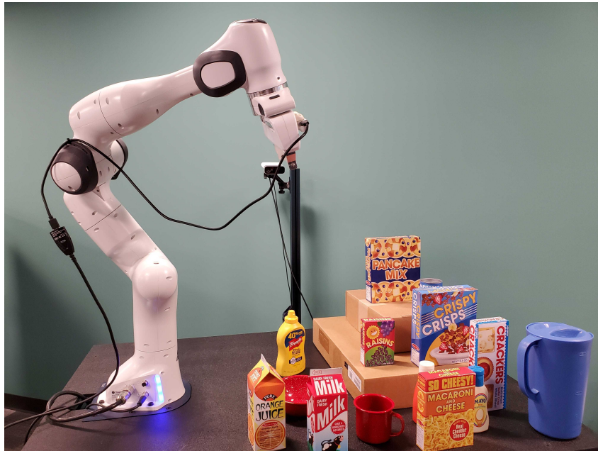
Figure 8: Real-world setup with multiple objects. The robot has an Intel Realsense D415 RGB-D camera mounted on its end effector at a known offset. We changed the scene geometry by positioning several large boxes.
