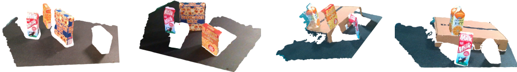
Figure 10: Examples of placement actions given individual snapshots of real-world scenes. In the top row, the robot was asked to move either the orange macaroni box to behind the milk (left), or the milk to the left of the macaroni (right), on a flat table. In the bottom row, the goal was to place macaroni (left) or juice (right) behind the milk; we added a cardboard box, which means that the object has to be placed off the table.
