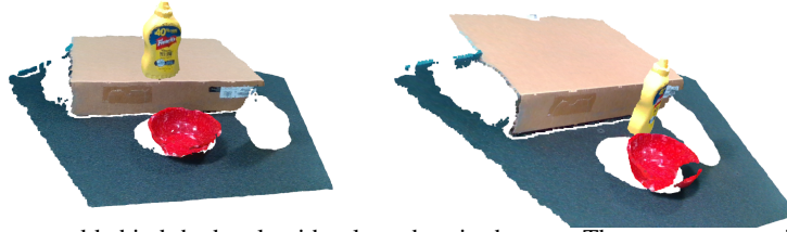
Figure 5: Placing mustard behind the bowl, with a large box in the way. There are two possible solutions to the problem: either placing the mustard on the table or placing it on top of the box. Our approach found stable placement positions in both locations.
