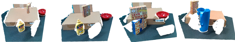
Figure 11: Some additional arrangement results for the “granola box” object. The planner finds a variety of poses, including stacking objects on top of one another, should that satisfy the specified predicate.
