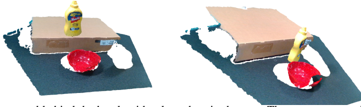
Figure 9: Placing mustard behind the bowl, with a large box in the way. There are two possible solutions to the problem: either placing the mustard on the table or placing it on top of the box. Our approach found stable placement positions in both locations.
