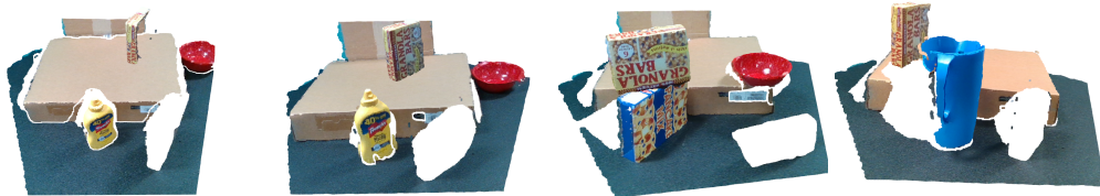
Figure 7: Some additional arrangement results for the “granola box” object. The planner finds a variety of poses, including stacking objects on top of one another, should that satisfy the specified predicate.
