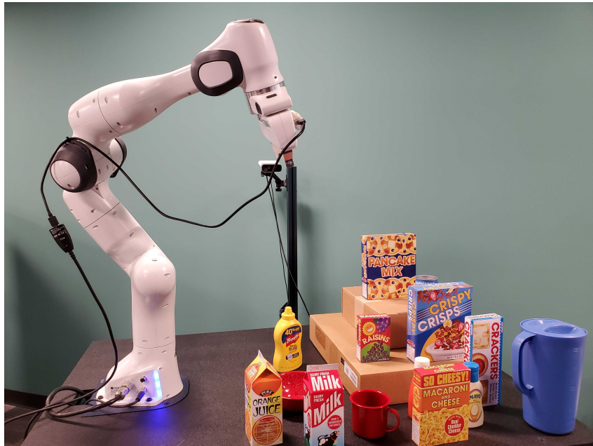
Figure 4: Real-world setup with multiple objects. The robot has an Intel Realsense D415 RGB-D camera mounted on its end effector at a known offset. We changed the scene geometry by positioning several large boxes.
