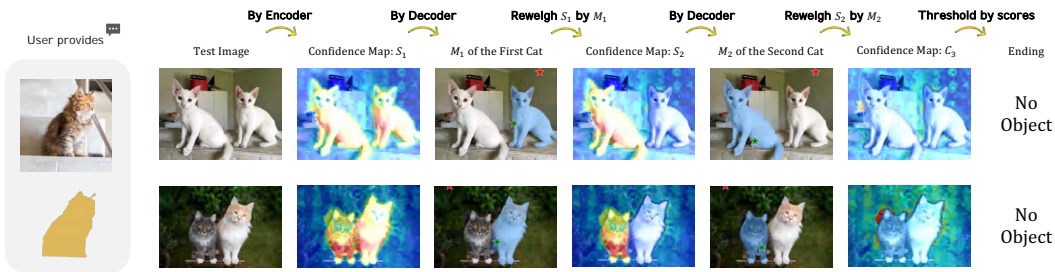
Figure 7: Segmenting Multiple Similar Objects in an Image. We adopt two strategies for PerSAM to simultaneously segment multiple similar objects: iterative masking and confidence thresholding. We denote the positive and negative location prior by green and red pentagrams, respectively.
