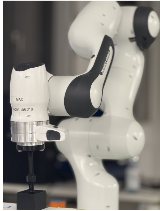
Fig. 3. Real-world screw insertion with gesture-based Cartesian control.
