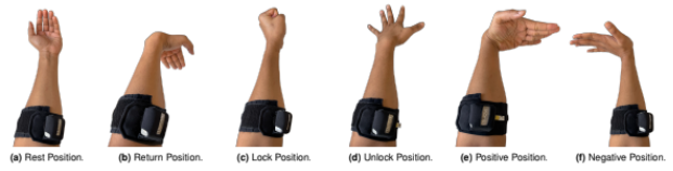
Fig. 2. Gesture set used in the interface: rest, return, lock, unlock, positive action, and negative action.
