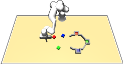
Figure 11: Inserting (T6) . Similar to T3, the Inserting task involves the robot pushing blocks to designated target zones. However, this task is more complex due to: i) the presence of three blocks and corresponding target zones, resulting in |\mathcal{B}| = 6 , ii) longer time horizons, and iii) the need for dexterous manipulations arising from additional constraints imposed by the gray barrier. The dataset comprises a total of 800 demonstrations, evenly distributed among the six behavior descriptors \beta .
