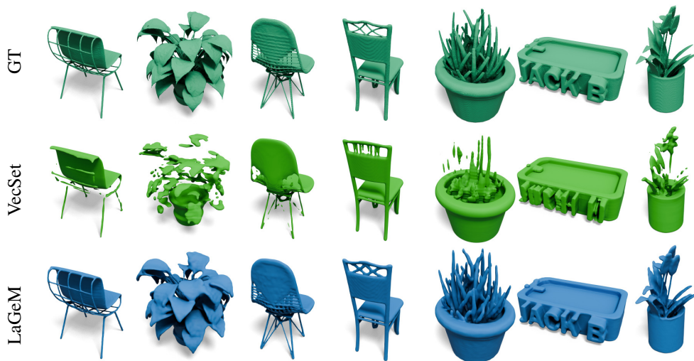
Figure 8: Qualitative Results on ShapeNet. We show autoencoding results on ShapeNet. We use VecSet as the baseline. Our model is capable of reconstructing detailed geometry, especially thin structures.
