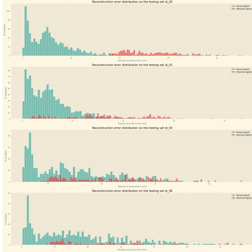
Figure 3: Histogram of reconstruction errors under normal and abnormal operation of machine id 00, 02, 04, 06.
