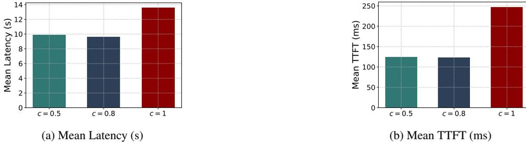
Figure 5: Comparison of mean latency and TTFT across different values of  $c$  ( $c = 0.5, 0.8, 1$ ) at a request rate of 14.
