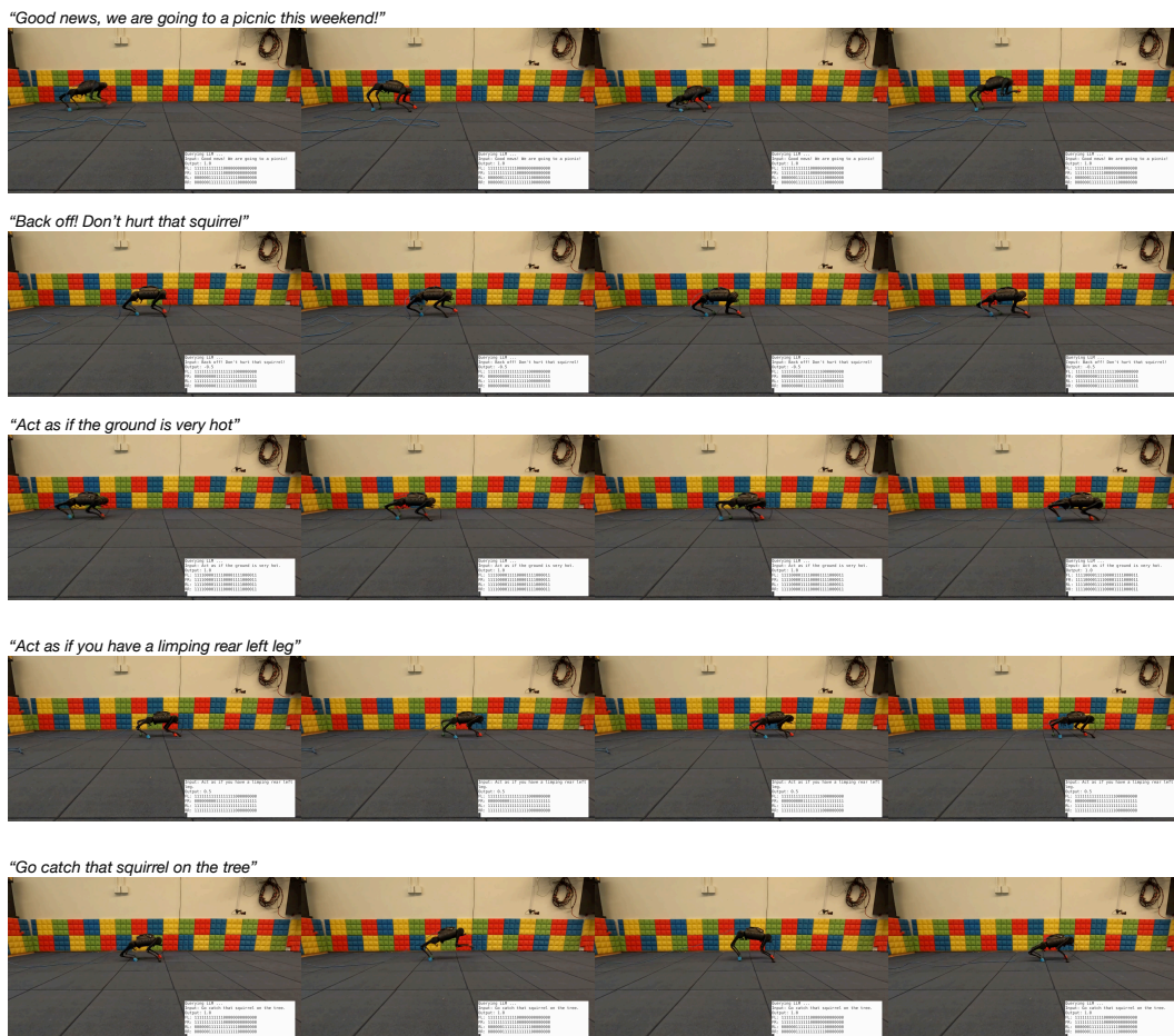
Figure 8: Images from the extended tests. We show the command for each test on the top-left corner on each row. LLM translated foot contact patterns are shown at the bottom-right corner in each image. Motions better viewed in the supplementary video.
