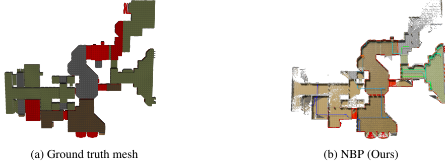
Figure 5: Failure case 1: Our method initially prioritizes the exploration of high-value areas, inadvertently neglecting regions of secondary importance. Thus, it results in incomplete reconstruction in the initial area of the beginning trajectory.
