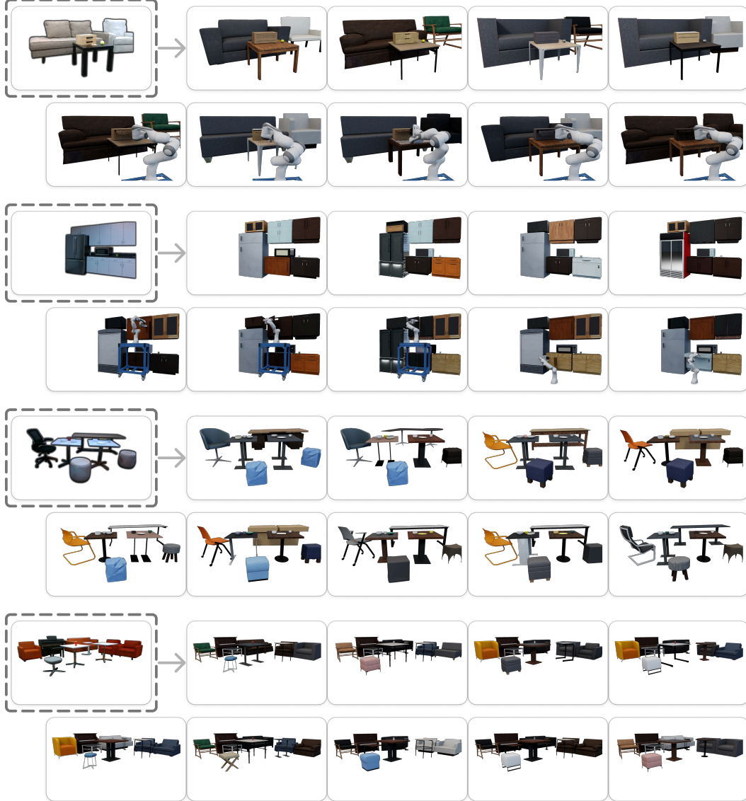
Figure 7: Qualitative ACDC real-to-sim scene reconstruction results. Multiple cousins are shown with a robot collecting demonstrations. Images cropped by dashed squares are input RGB images.
