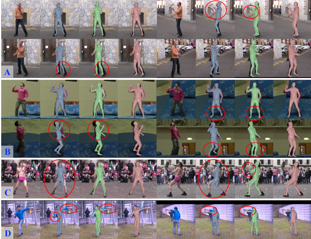
Figure 1: Qualitative comparison between Liang [15] (blue), post-hoc multiview fusion (average of body model parameters across views) of SPIN [9] (green) and ours (pink) on Unstructured VBR [1] (A, B, C), and MARCOI [4] (D). Each block shows multiview images of the same subject taken at the same time and reprojections of the 3D mesh reconstructed by each method. Red circles highlight regions with wrong predictions.
