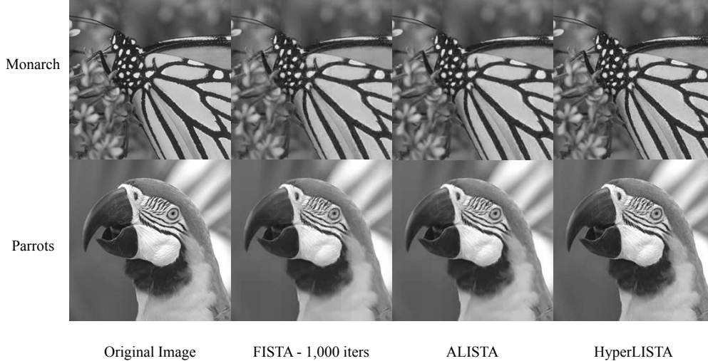
Figure 9: We visually present the recovered images using 1,000 iterations of FISTA and 16-layer ALISTA and HyperLISTA. We can see that HyperLISTA has much less artifacts at the boundaries of patches.
