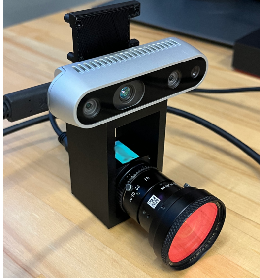
Figure S2: Example of rigidly-attached event camera (Prophesee Gen3.1 VGA) and depth camera (Intel Realsense D435) used to gather events batches and depth images for approximate post-processing calibration and time synchronization, for use in fine-tuning perception backbone from Figure 2. Note that an IR filter is used on the event camera lens so that we may enable the infrared emitter on the D435 for more-accurate indoor depth images.
