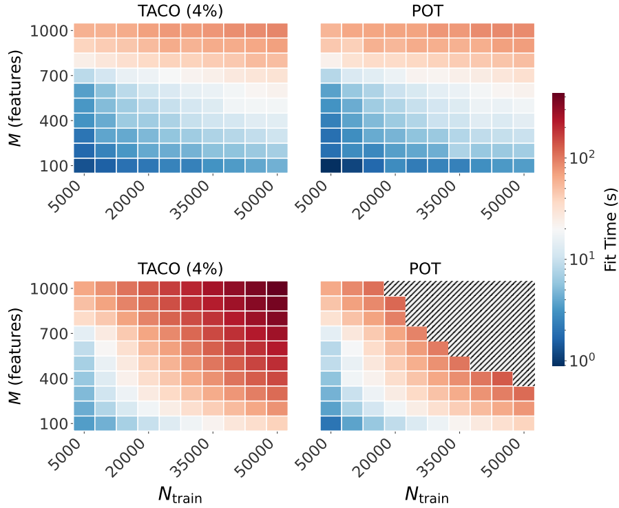
Figure 10. Fit Time Heatmap. Top: Fit times for TACO and the Predictor Transformer, without using KV caching. Bottom: Fit times with KV caching. Black shaded regions indicate out-of-memory errors.
