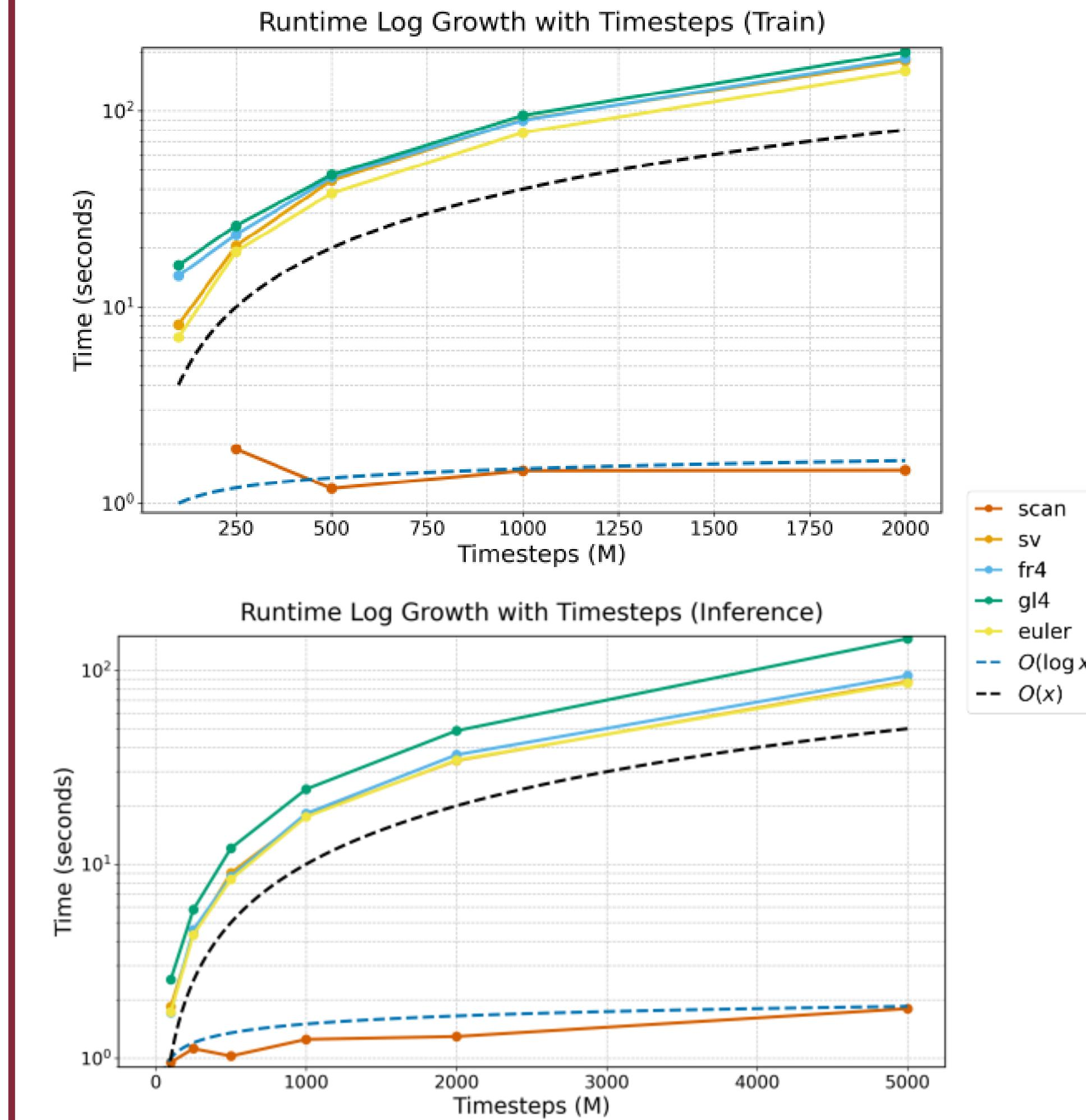
As seen in the graph, our model shows log-scale complexity along the timescale, offers a scalable path for fast neural simulators in large-scale physics.
